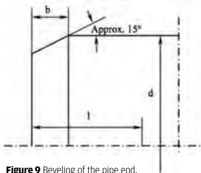
**Figure 9** Beveling of the pipe end.
