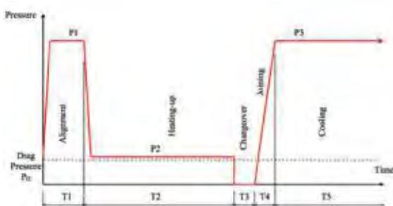
Graphic 2: Process stages of butt welding
