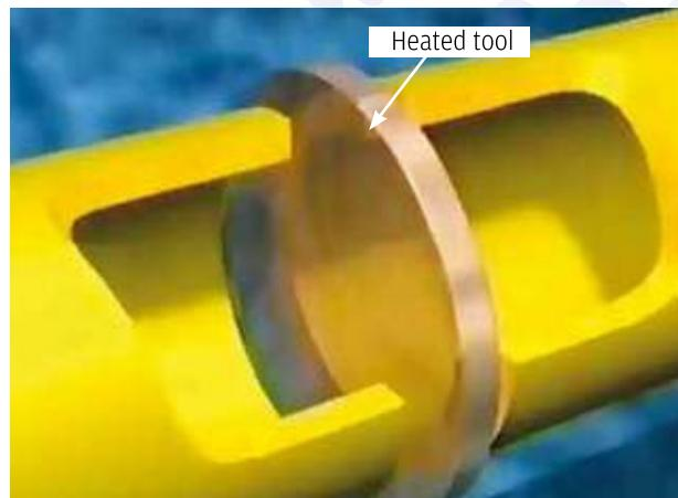
Figure 3: Inserting the heated tool
