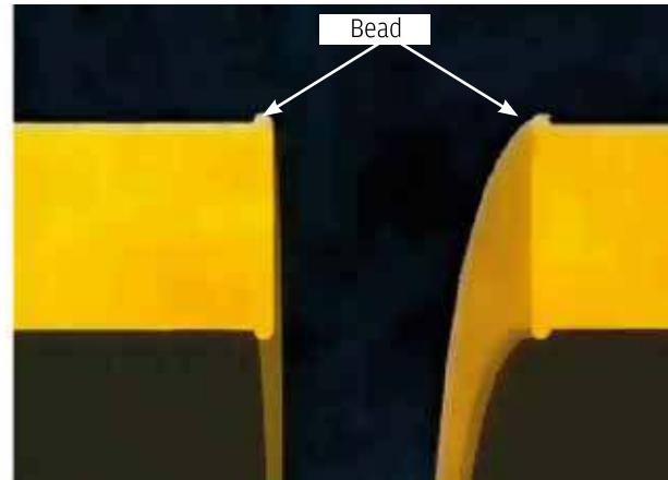
Figure 4: Bead shapes during and after alignment
